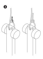
Bring the lead up through the loop from underside of the loop
