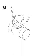
Form a loop with the lead passing over the line
